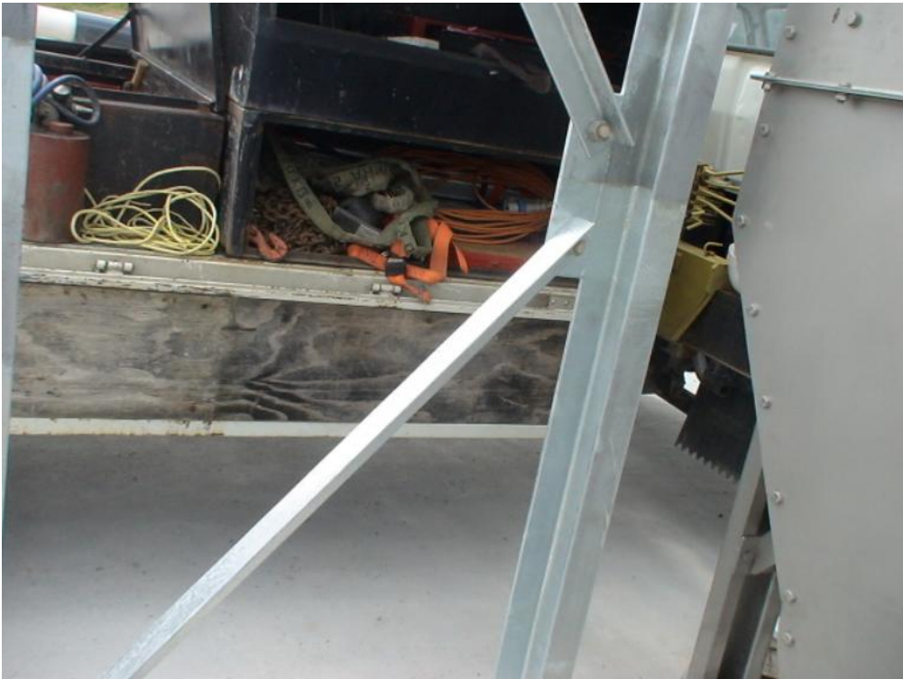
Figure 1.8 — Noise Source 08: Structural beams. Fix: Fill hollow beams.
